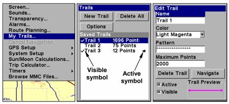
Sequence for saving a trail and beginning a new one. My Trails command (left). The Trails Menu (center). The arrow to the right of Trail 3 indicates the trail is "active," and the check to the left indicates the trail is visible on the map display. The third figure (right) shows the Edit Trail menu, with the Name command selected.
